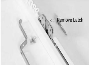
Bring the loose carrier together and join with the latch piece. Reattach the master carrier to both pieces.
