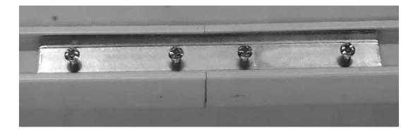
Loosen the screws on the master carrier and remove latch.
