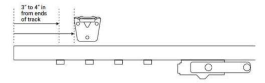
Measure the width of the track and mark the two end brackets approximately 3"-4" in from ends of the track. Evenly space the remaining brackets and place corresponding marks. We also recommend that the remaining brackets be placed every 16-24" (We recommend placing brackets on studs, if not possible use heavy duty anchors.)
