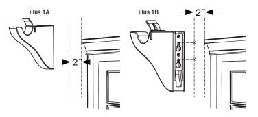
3. If using plastic expansion anchors, pre-drill holes using 3/16" drill bit. If drilling directly into a stud or wood trim, pre-drill holes using 3/32" drill bit. Attach the mounting screws into the mounting surface so that the head of the screw forms a gap of approximately 1/8" between the screw head and mount surface (see illus 1C).
