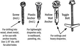
Begin with the two outside ends. Determine the desired height and width based on the curtain measurements. Be certain to make the appropriate allowance for the decorative hardware. It is recommended that the brackets be installed approximately 2"-4" beyond the window frame (see illus 1A).
