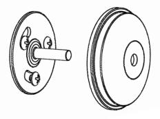
Tips for Successful Installation Securely attach all Holdbacks to the mounting surface. If you do not locate and install into wood studs. Use the proper wall fasteners and / or plastic anchors designed for your particular mounting surface (fasteners are included). When drill into metal, use self-tapping screws (not included).
